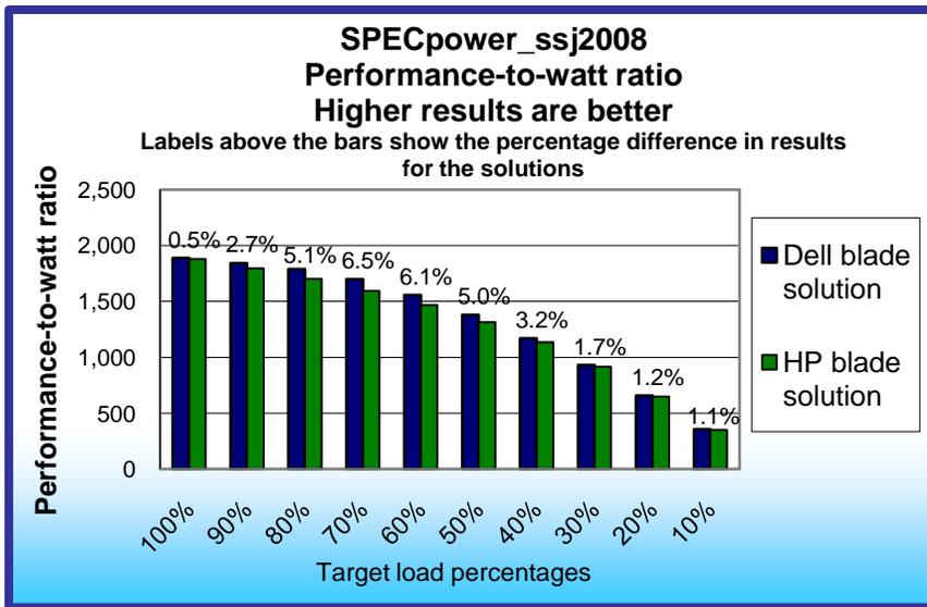
Figure 4: Performance-to-power ratios (ssj\_ops/watt) reported by SPECpower\_ssj2008. Results include the Overall ssj\_ops/watt result and the ssj\_ops/watt results for each of the measurement intervals. Higher results are better.
