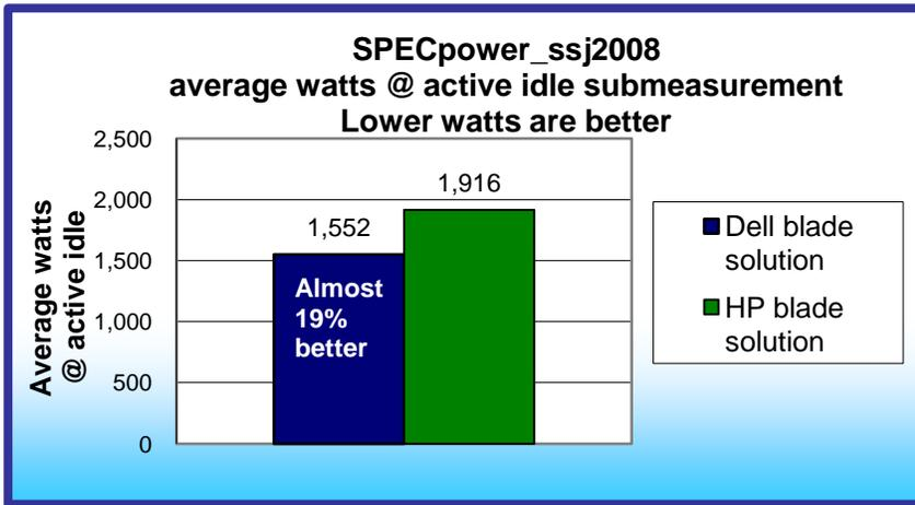
Figure 2: Idle power results of the blade server solutions using the SPECpower\_ssj2008 benchmark. During the idle test, the blades run without any transactions scheduled by the workload software. Lower idle power is better.
