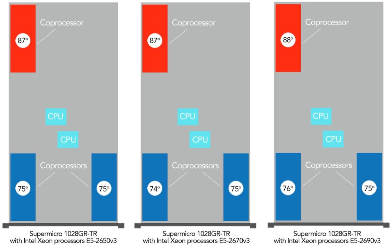
**Figure 4: Coprocessor and CPU placement in the two servers we tested showing sensor temperatures with multiple Intel Xeon processor configurations. Lower temperatures are better.**
