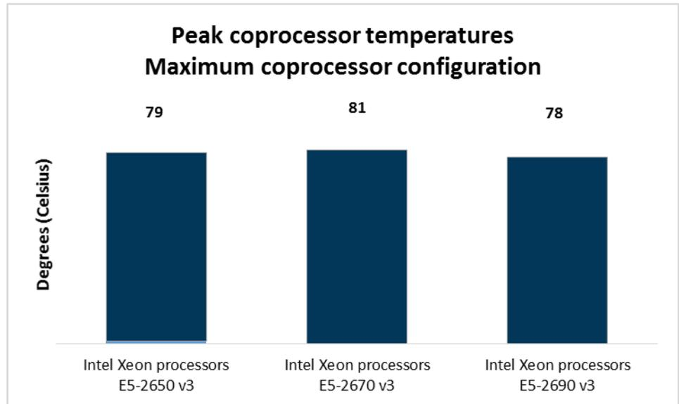
If your organization needs the power of coprocessors to run graphic-heavy design applications or complex scientific simulations, the Dell PowerEdge C4130 can provide the hardware to support your demanding workloads. Keeping the silicon of coprocessors at a reasonable temperature, as the PowerEdge C4130 did, could extend the lifetime of the chips, while reducing diminished performance and power inefficiency.
