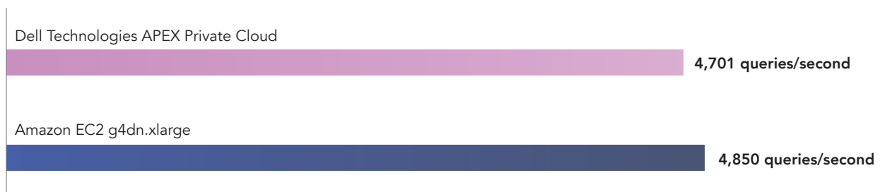
Figure 2: The queries per second that the machine learning VM of the APEX Private Cloud solution and EC2 g4dn.xlarge instance handled during the image classification workload we used in testing. Higher is better. Source: Principled Technologies.
